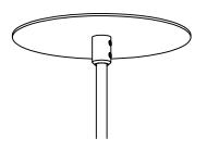
Mounting Option Power 1-5 Octagon Box (By Others) Installed in drywall, wood or concrete ceiling
